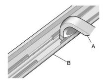
Levers must still be in the forward up position. Move the front crossrail forward beyond the cut-out area (B). For the rear crossrail, slide the crossrail assembly (A) rearward until the entire crossrail support is in first position beyond the channel cut-out area (B).
